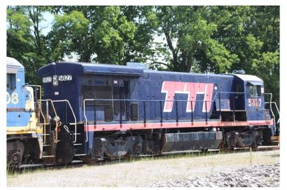
TTI 5827 is a General Electric B36-7, that was obtained from CSXT. Previously the locomotive served on the Seaboard System Railroad. She was obtained by SBD through the merger with the Seaboard Coast Line, where she was No, 1797. The locomotive appears in an earlier TTI paint scheme
