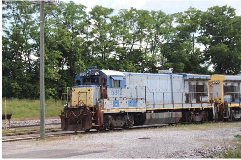
The photos show TTI 5812 and TTI 5808, both General Electric B36-7 locomotives. They were purchased from CSXT for use as a spare part source. Both are former Seaboard System Locomotives. The photos show clear reminants of CSX paint.
